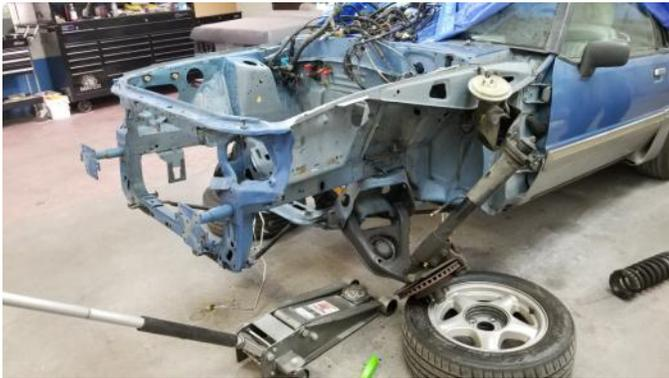
Step 1 was removing the front bodywork, suspension, and steering. Then the entire front end and subframe was prepped and painted in Bright Regatta Blue Metallic to match the exterior. The original AOD transmission was also sent out for a complete rebuild and upgrade to handle the additional planned horsepower.
